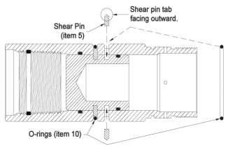
**2.3** Install an O-ring (item #8) on the Cap (item #3) and apply grease to the O-ring. Insert the Cap into the Body until it's seated in the tool and the 4 shear holes are clear of the Cap lip. Insert the 4 Brass Shear Pins (item #6) into the holes, securing the cap in place. Install the O-ring (item #7) into the groove on the pin-end of the Body.
